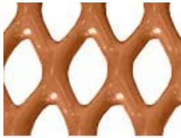
Figure 6.4 A photo showing an example of vinyl-coated metal flooring surface used in a study by Wilson et al. (1998).
