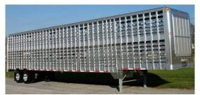
Figure 6: Tandem Axle Double-Deck Trailer (Source: Eby Inc.)
